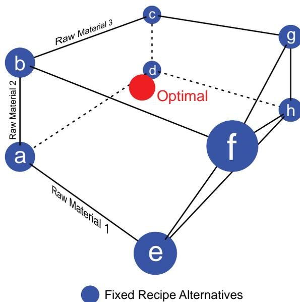
Figure 2: LCF optimized line uses 3 materials to create a 3-dimensional control space
