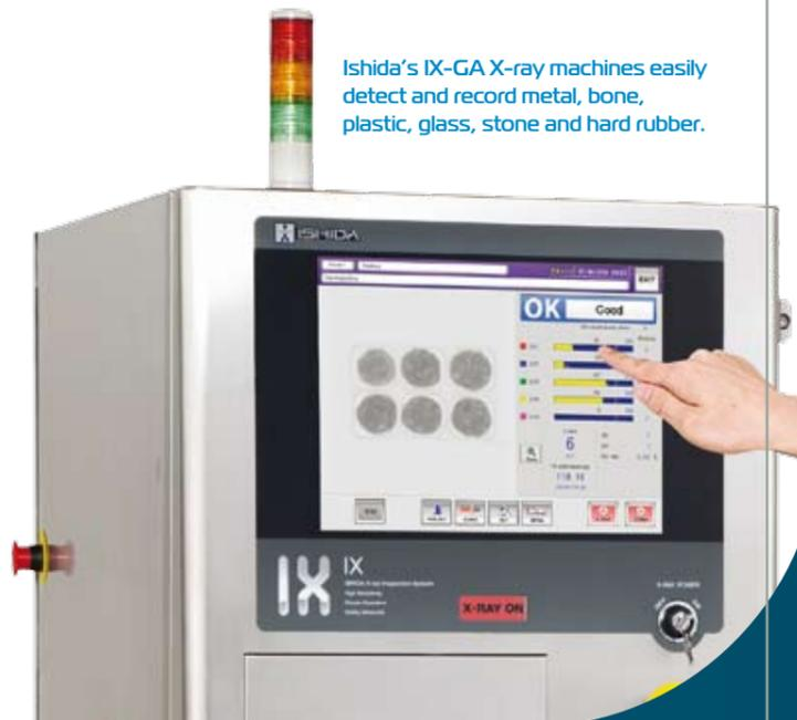
**Ishida's IX-GA X-ray machines easily detect and record metal, bone, plastic, glass, stone and hard rubber.**
